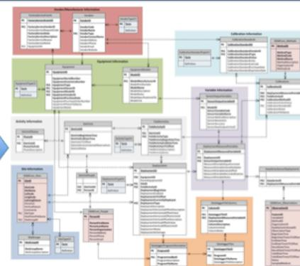
**Sensors Extension.** The Sensors Extension permits information about individual sensors, deployments, and the associated time series to be recorded and managed.
